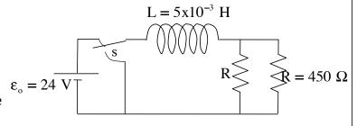
be a steady-state current through the inductor and the resistors. As there is no induced EMF across the inductor, it will not be a player in impeding current flow and the net current will be:
